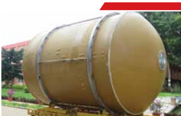
The heaviest Semi-Cryogenic propellant tank (SC120- LOX) ever fabricated by HAL was delivered to Indian Space Research Organization (ISRO) on October 5, 2021.
